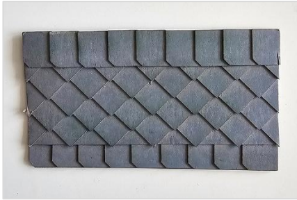
P002 – Eternite covering
