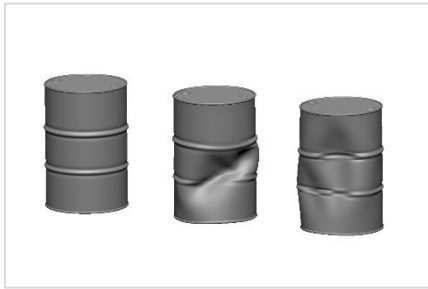
C078 – Barrels 200l (damaged)
